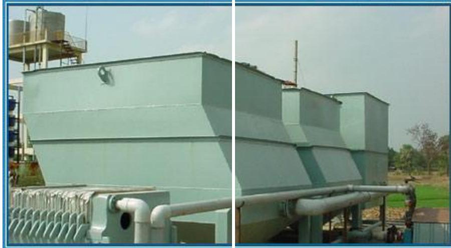
Effluent from leather industries contain different types of contaminants which generally includes chrome and other toxic chemicals. WETCO effluent treatment plants comprises of units for primary and secondary treatment of the effluent. The treatment is complex and requires seamless integration of different process. We have successfully installed various plants for leather processing and tannery effluent treatment.
