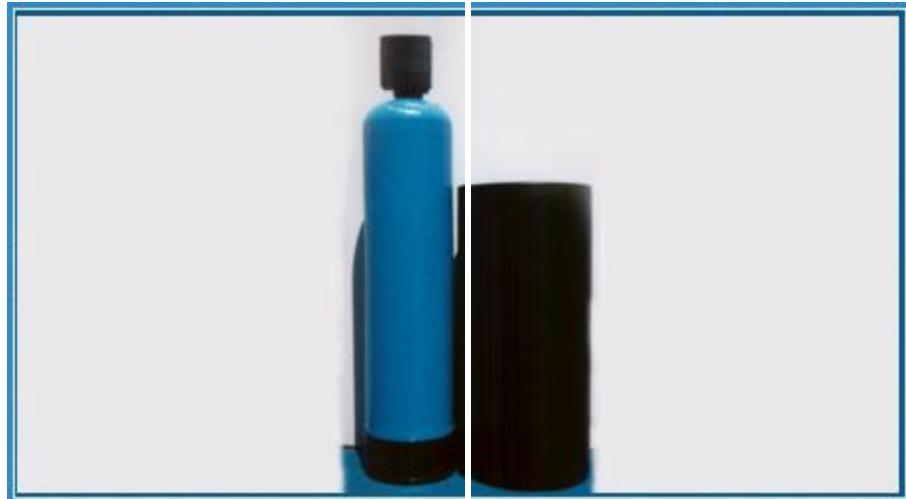
Auto regeneration softening system from Impex utilizes the proven ion exchange technology to remove hardness from water. The regeneration valve is adapted for automatic activation of ion exchange resin to replace calcium and magnesium ions. Our compact unit for water softening is available with PLC for easy operation. Auto regeneration softening system can be automatic semi automatic or largely manual as per the client's demand.
